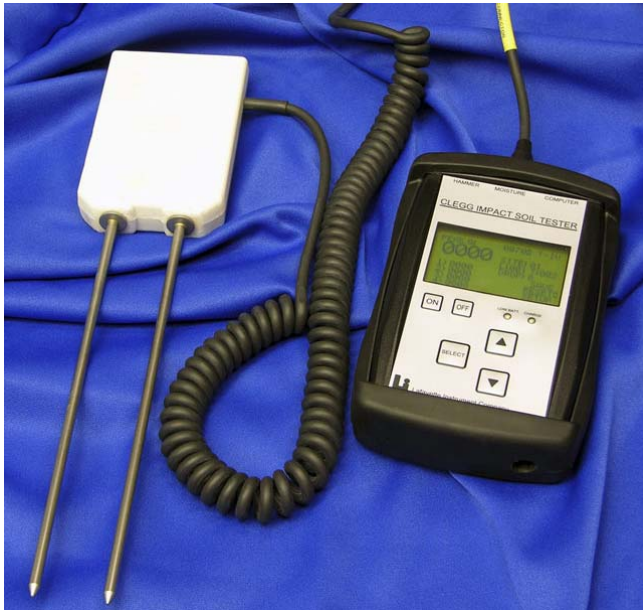
Figure 12 -Campbell moisture sensor (CS620) connected to the readout box
