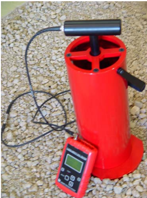
Figure 10- Final prototype with improved hammer drop and reduced weight
