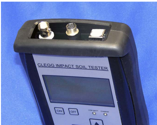
Figure 13 - The moisture sensor (CS620) connection to the readout box
