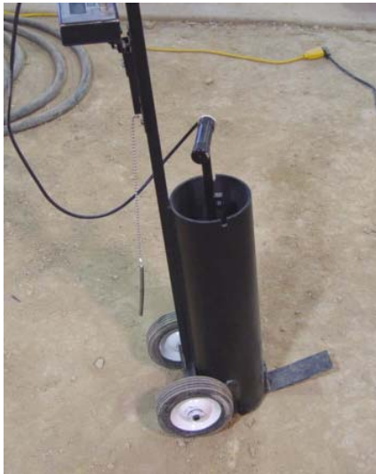
Figure 2 - The 10-Kg Clegg Hammer used in Phase-One of the study
