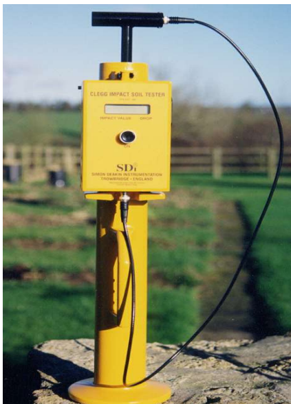
Figure 3 - Early version of the Impact Soil Tester Device
